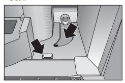
Clean the surface the water container sits on thoroughly, taking special care to clean the recesses properly.
